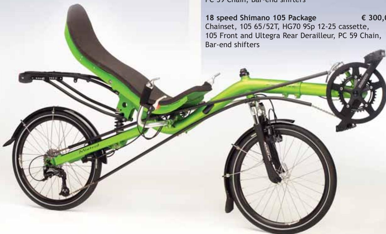
In the Mistral Deluxe, the rear suspension is concealed within the frame. The same high-end design of the wishbone rear end of the Mistral Deluxe is also used for the Seiran, Fujin and Taifun.
