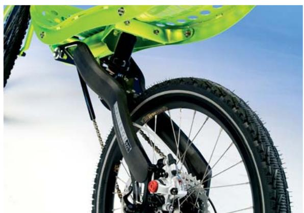
The carbon rear end is the *piece de resistance*: stiff, strong, and very light. Traditionally an expensive handcrafted process, we have designed our carbon rear fork to be injection moulded by machine. By using aerospace techniques, we keep material, production methods advanced while keeping the price low.
