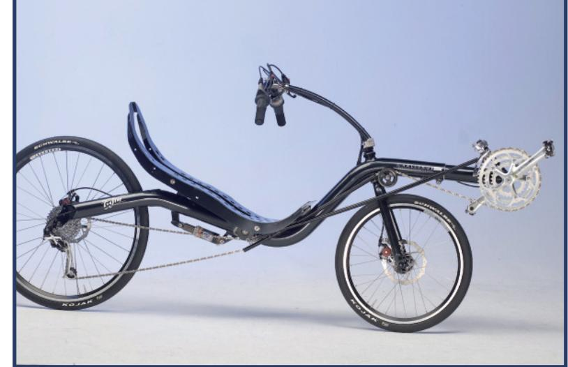
The Fujin-sport combines the comfort of a suspended recumbent with the pedegree of a low-racer. With its 26" rear wheel, 35cm seat height and 123cm wheelbase, the Fujin is perfect for going, really far, really fast. For riders seeking the ultimate comfort racer, we offer the Fujin with the Challenge front suspension system. For the greyhounds out there we offer a hardtail racing version.
