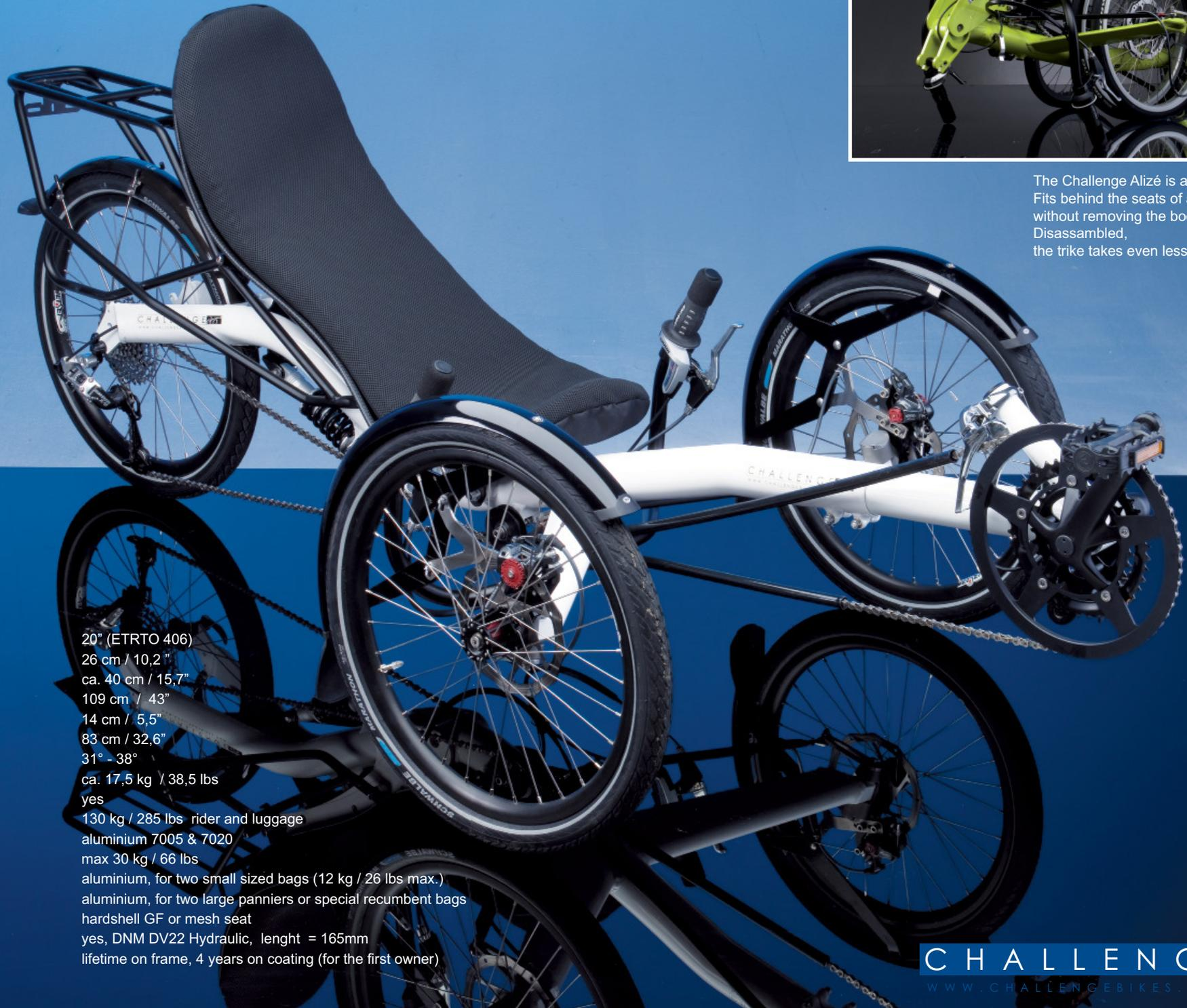
The Challenge Alizé is a folding trike. Fits behind the seats of a Smart car without removing the boom. Disassembled, the trike takes even less space.
