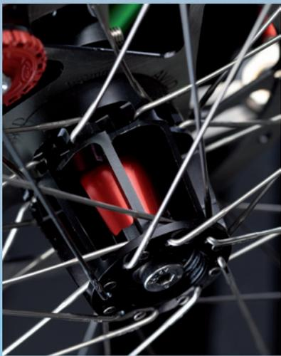
Challenge Trike hubs are loaded with innovation. A stylish and strong tapered shape with cut-outs to save weight and also give a look “inside.” 32 traditional style spokes for easy service and oversize inside bearings give better heat transfer and long life under high side load cornering forces.
