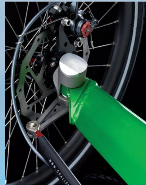
A cast stainless steel housing pillar enhances structural integrity while attractively concealing the engineering in a compact space.
