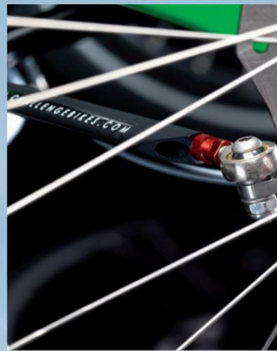
Aero profile tie rods feature clean internal cable routing, and the double thread arrangement gives easy toe-in adjustment at the ends. Elegantly finished in anodized black.
