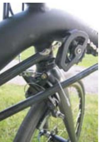
we had a SRAM model) runs through slippery plastic guide tubes, which also keep your legs clean. I should own up to getting the return-run chaintube the wrong side of the tension-side one for the photos, so don't go assembling yours like that. The power-side idler pulley is actually a large-diameter gear cog, reducing transmission losses and keeping it all quiet.
