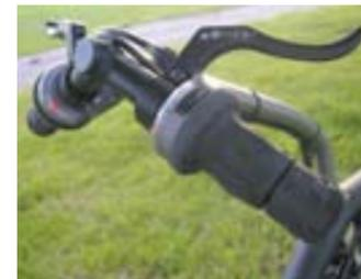
**Compact bars, with the four cable runs neatly routed down below the stem**
