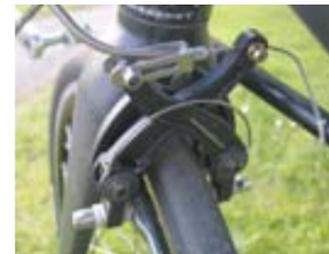
**Challenge's own-design brakes fit neatly behind the carbon forks**
