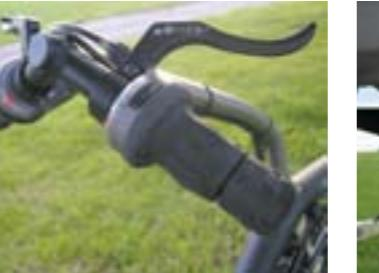
**Compact bars, with the four cable runs neatly routed down below the stem**
