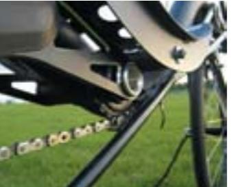
**The main drive-side chain roller is really a toothed sprocket**
