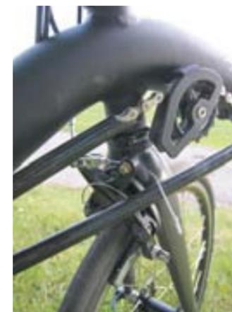
the walls thinner on the tube sides, and thicker on the top and bottom...
