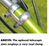
ABOVE: The optional telescopic stem employs a very neat clamp to secure the length adjustment. Perhaps the handlebar clamp could be made prettier to match!
