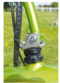
ABOVE LEFT: The stem folds on this stainless steel bracket, with a bolt to set its resting angle. Ours needed a touch of threadlock!
