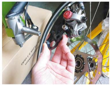
**ABOVE:** The disk brake calliper is mounted to a separate black anodised aluminium bracket. To re-assemble, the caliper slips over the brake rotor and the whole thing is slid onto the axle and secured by an Allen bolt.
